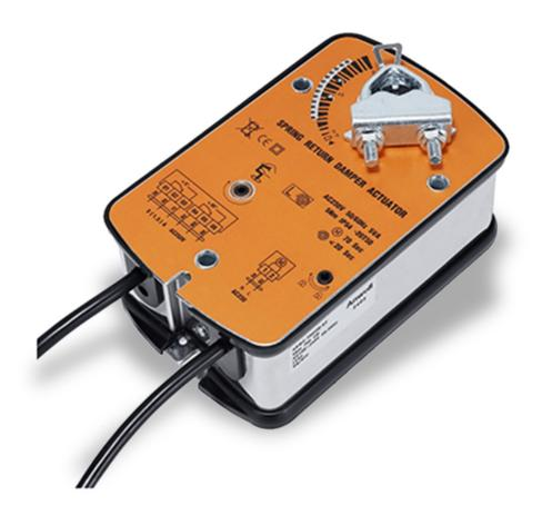
SRA81 series electric damper actuators adopt imported DC motor/brushless motor to provide power with torques of 5NM. It is widely used in building ventilation felds, which can realize mechanical reset when power off and electric start, providing more than 30000 times of repeated action.
